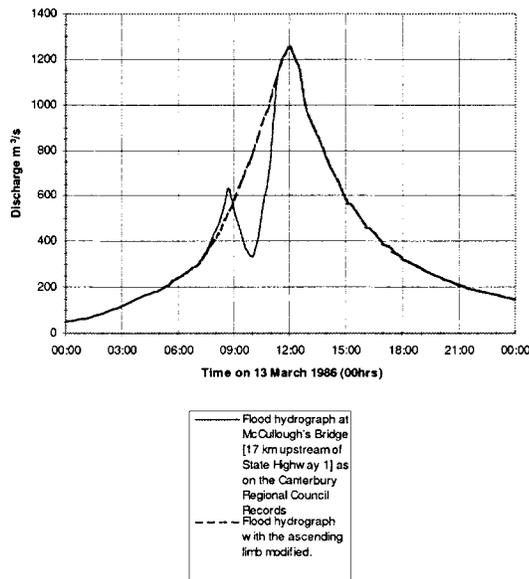
FIG. 4. Hydrograph of 1986 Flood
