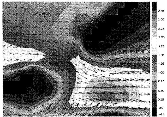
FIG. 9. Velocity Vectors and Unit Discharge Rates Used to Estimate Outflow for Breach 5 of Fig. 8
