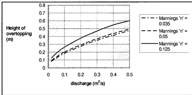
FIG. 7. Manning's *n* Effect on Overtopping Discharges
