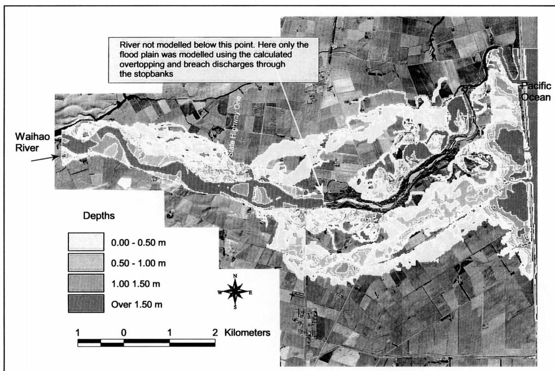
**FIG. 11.** Modeled Extent of Flooding March 1986 Flood
