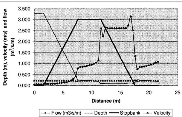
FIG. 6. Levee Overtopping Profiles—0.2 m<sup>3</sup>/s/m
