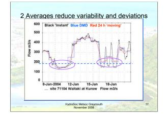
The right-hand oval shows both DMD and 24-hr moving average flows above minimum while the 'instant' flows go below it. It is less marked, but the left-hand oval also shows average flows above minimum for different times when the 'instant' flows are below it.
