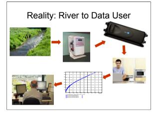
Real river, to level logger, to wireless network, to database manager office, via rating [level to discharge], to user.
