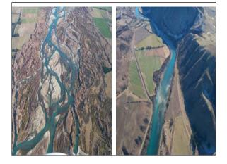
It is little use trying to measure flow in the braided lower river by conventional means. The recorders are back up above Kurow in a single channel and at the Waitaki Dam.
